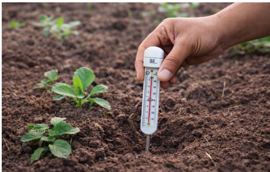
Figure 3. Use of a manual soil thermometer during field assessment
