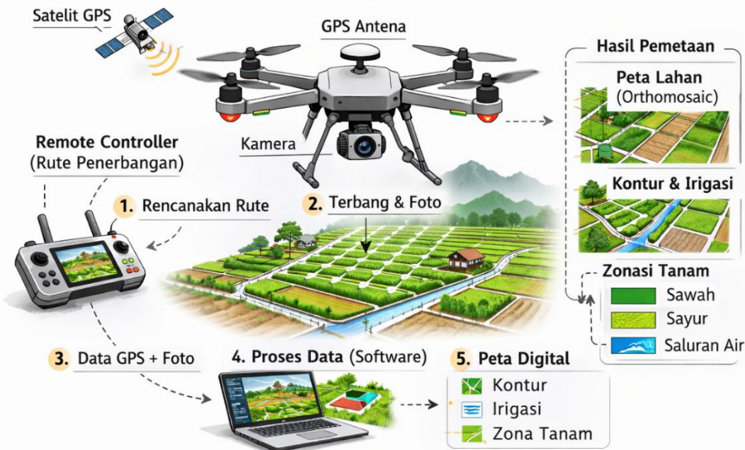
Figure 2. How the drone works for mapping
